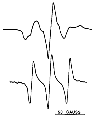
Figure 3. The derivative epr absorption curves of dilituric acid in solid (upper tracing) and melt (lower tracing).
